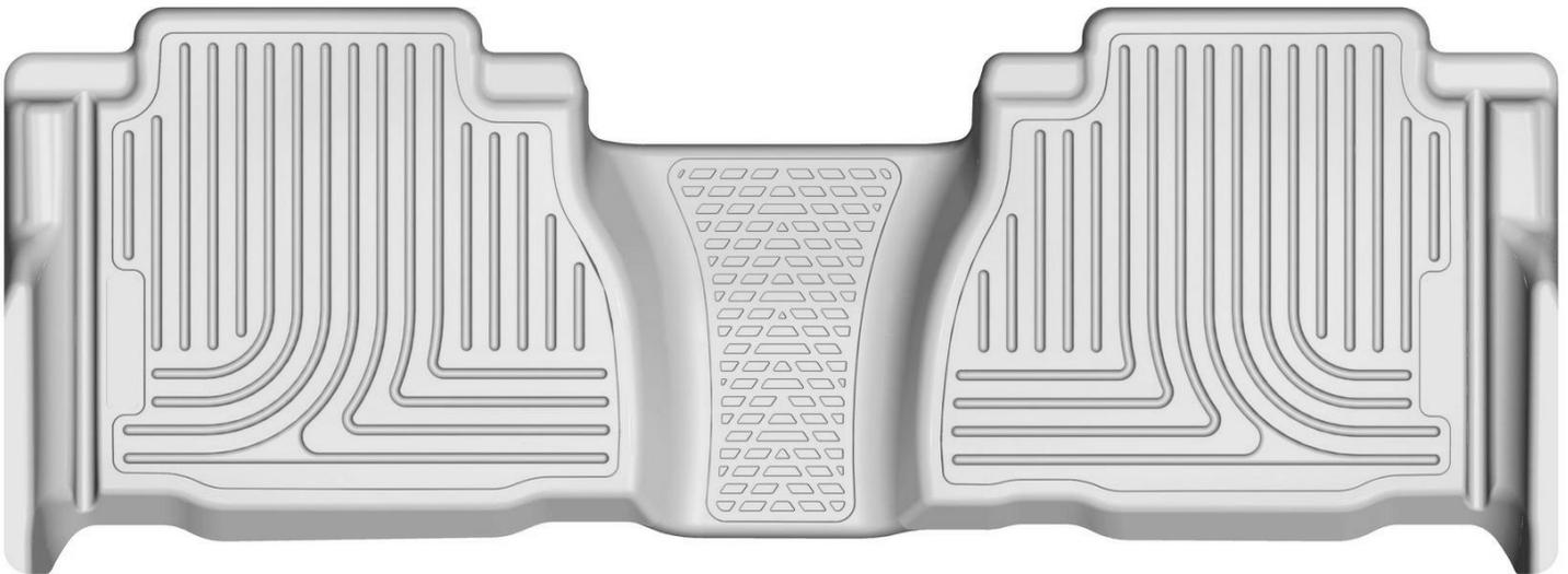
TO EASE INSTALLATION OF YOUR TUNDRA SECOND SEAT LINER, MOVE THE FRONT SEATS TO THEIR MOST FORWARD POSITIONS AND FOLD UP (DOUBLE CAB) OR SLIDE BACK (CREWMAX) THE SECOND ROW SEATS. WITH THIS DONE, INSERT THE LINER IN VEHICLE ANGLING THEM SO THAT THE FRONT EDGE OF THE LINER IS SEATED INTO PLACE FIRST, THEN, LOWERING THE REAR EDGE. ONCE THE LINER IS INSTALLED, REPOSITION THE FRONT SEATS AS DESIRED.
