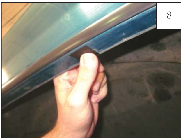
Remove flare. Center a supplied Tab (MT1-0002) over the marks made in Step 6, aligning edge of tab with inside edge of fender lip (tab may extend over outside of fender).
