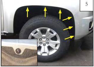
Using a T-15 torx bit, remove six factory fasteners from wheel well. Retain for bracket installation.
