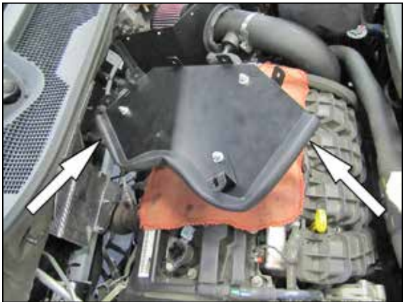
28. Install the 22" long edge trim onto the air box lid as shown.
