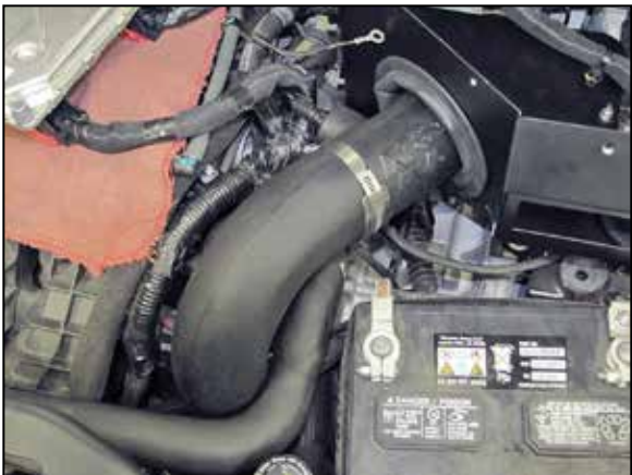
23. Install the K&N® intake tube into the silicone hose at the throttle body and then secure the intake tube with the provided hose clamps.
