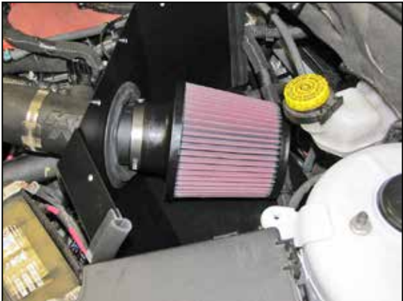
24. Install the K&N® air filter and secure with the provided hose clamp. NOTE: Drycharger® air filter wrap; part # RU-4990DK is available to purchase separately. To learn more about Drycharger® filter wraps or look up color availability please visit http://www.knfilters.com ®.
