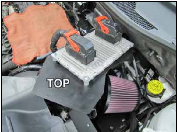
27. Secure the ECU and mounting bracket (083171) and ground strap to the air box lid using the provided hardware as shown.
