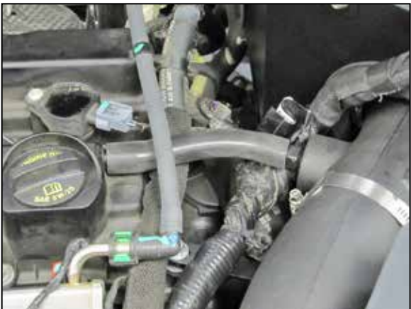
30. Install the provided crank case vent hose onto the valve cover port and then connect the open end to the fitting installed into the intake tube as shown. Trim and adjust as necessary to prevent collapsing of the hose.
