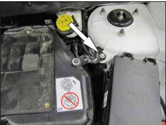
7. Remove the bolt securing the air box mounting bracket to the inner fender.
