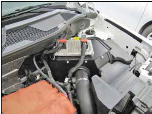
29. Secure the heat shield lid to the heat shield and factory air box mount using the provided hardware. NOTE: The wiring harness will need to be adjusted to allow the ECU and lid enough movement to be secured onto the heat shield. Disconnect the harness anchors from the attaching posts on the intake manifold, valve cover and engine. After the lid a ECU are secured to the heat shield, adjust the mounts on the harness and resecure the harness onto the valve cover and intake manifold.
