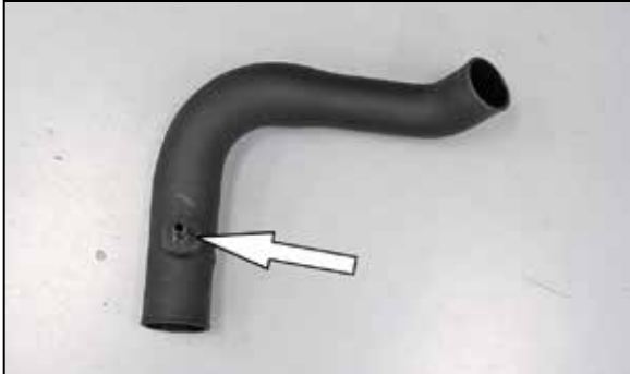
19. Install the provided vent fitting into the K&N intake tube as shown.
