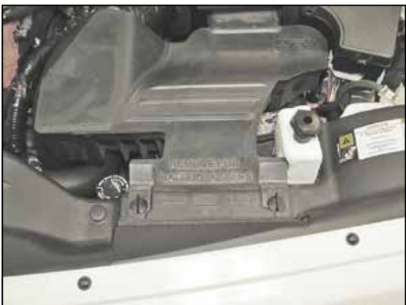
26. Install the fresh air intake scoop into the heat shield and then secure it to the core support with the factory clips.
