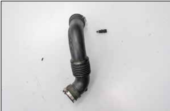
21. Remove the inlet air temperature sensor from the factory intake tube.
