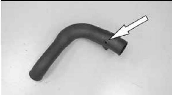
20. Install the provided grommet into the K&N intake tube as shown.
