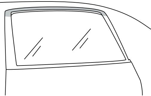
Remove tape liner from front and rear flanges. Peel back 2" of tape liner from each end.
