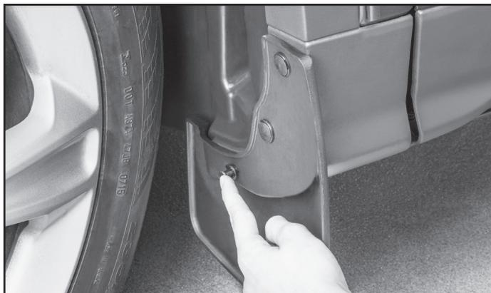
**8** Insert the supplied rivet into the bottom hole of the MudFlap. Push in the center core of the rivet firmly until flush with the outer portion of the rivet, it may take more force than the top rivets.
