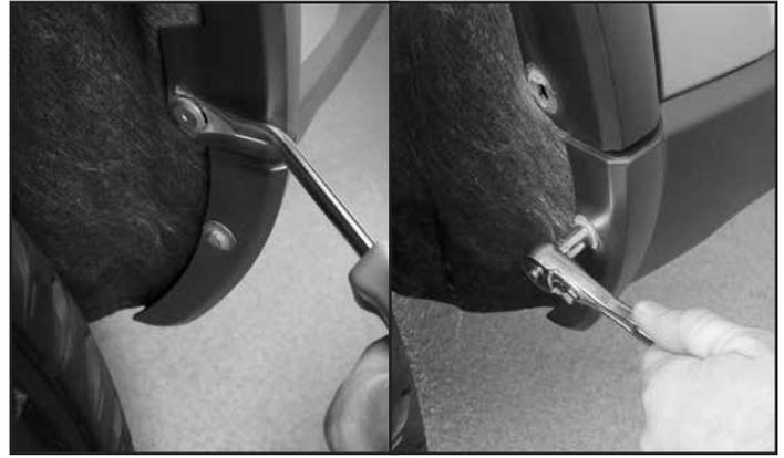
**4** Remove the factory plastic rivet with the trim clip remover. It will not be reused. Next, remove the factory screw with a ratchet and appropriate sized socket and retain for later use.
