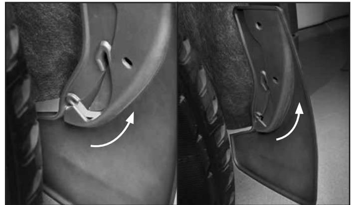
**6** Put the inner fender liner back in place. Then, using the MudFlap marked "LH," position it in between the inner fender liner and plastic edge of the fender, slide up and into position to align with the appropriate holes in the fender.
