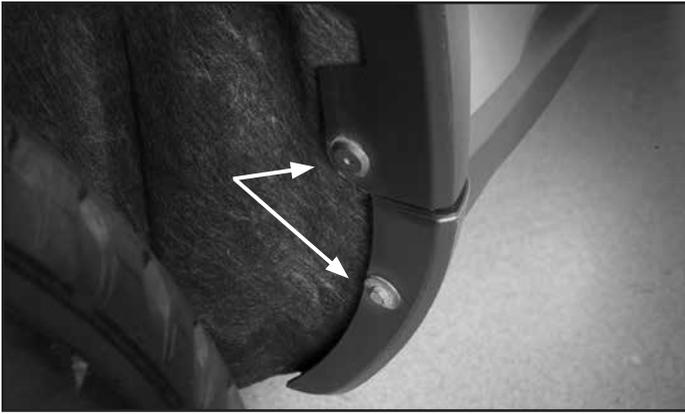
**3** Locate the (1) factory plastic rivet and (1) factory screw as indicated.
