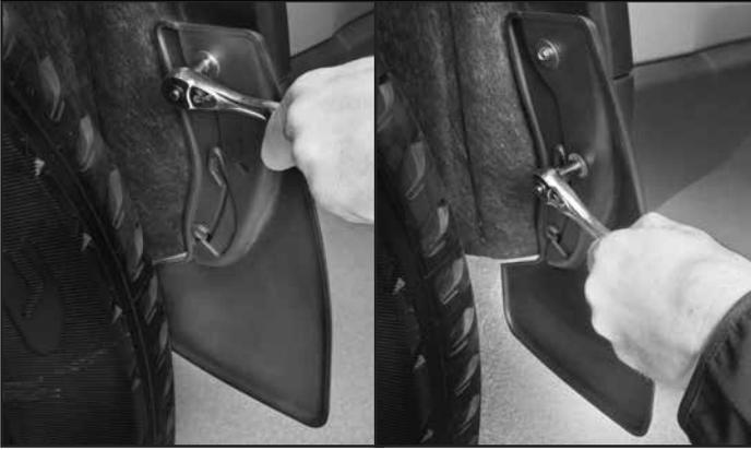
**7** Using the ratchet and appropriate socket, install the supplied screw and washer into the top hole of the MudFlap to a snug fit. Next, install the factory screw and washer into the bottom hole of the MudFlap to a snug fit. With the MudFlap aligned and pressed firmly against the fender, tighten each screw.
