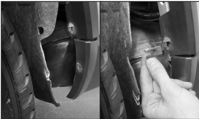
**5** Pull the inner fender liner out from the bottom of the fender. Next, install (1) supplied U-Clip by pulling the plastic fender back and pressing it on the steel fender as shown.
