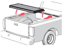
Center the cover side to side with the tool box. Unfold the cover fully and adjust position over the truck bed for proper front (cab)/
