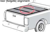
Carefully refold the cover without shifting its position on the truck bed.
