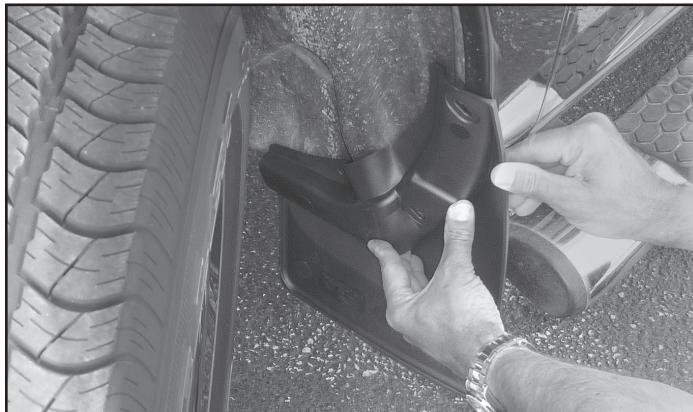
**5** Place the MudFlap marked "LH" in place on the fender. Line up the holes in the MudFlap with the holes in the fender lip and the wheel well liner behind it.
