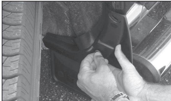
**6** Insert the previously removed fasteners through the MudFlap and fender lip, then thread into the clip on the wheel well liner. Do not tighten at this time.
